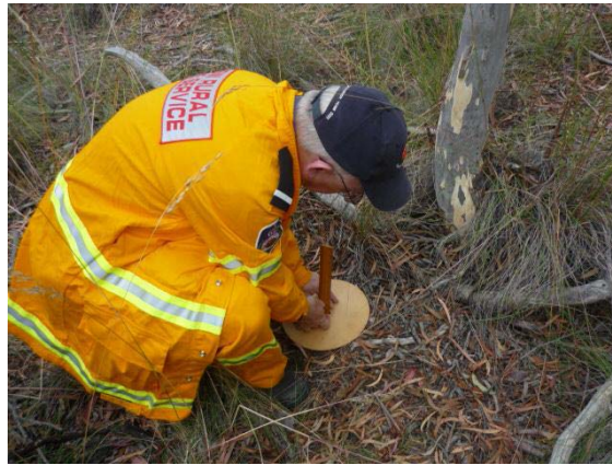
Deputy Captain Cliff Spong measuring the depth of fine fuel including leaf litter build up to determine fuel loading, ie tonnes per hectare, in the area.
